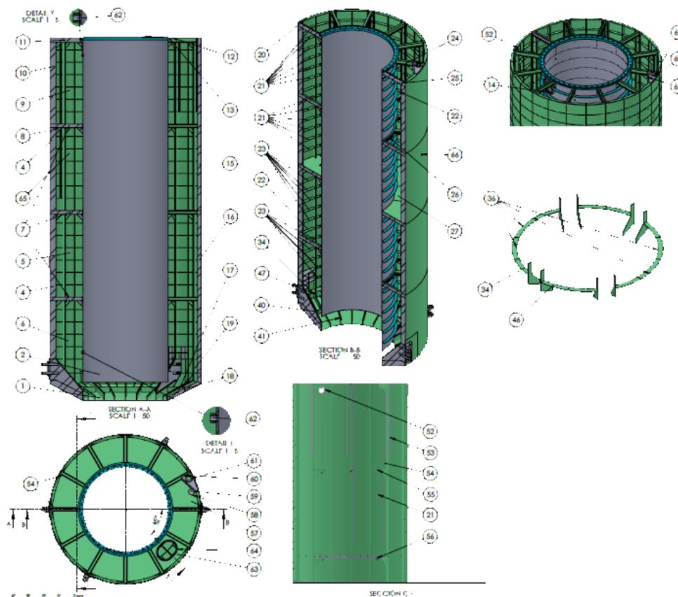
Figure 3. OCEANTEC oscillating water column floating device
