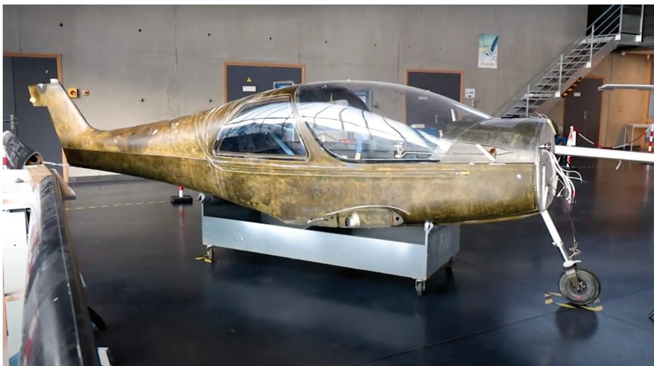
that match a real part's dimensions, and are sturdily manufactured with BigRep's affordable PLA filament. Because of the parts' added strength, POLYAERO's students are even able to include weights that further serve the realistic illusion they've created.
